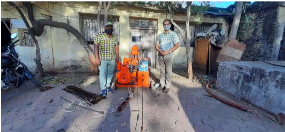
Photo 10: Kamrodder machine (1hp) for drain and pipe cleaning at Taloda
